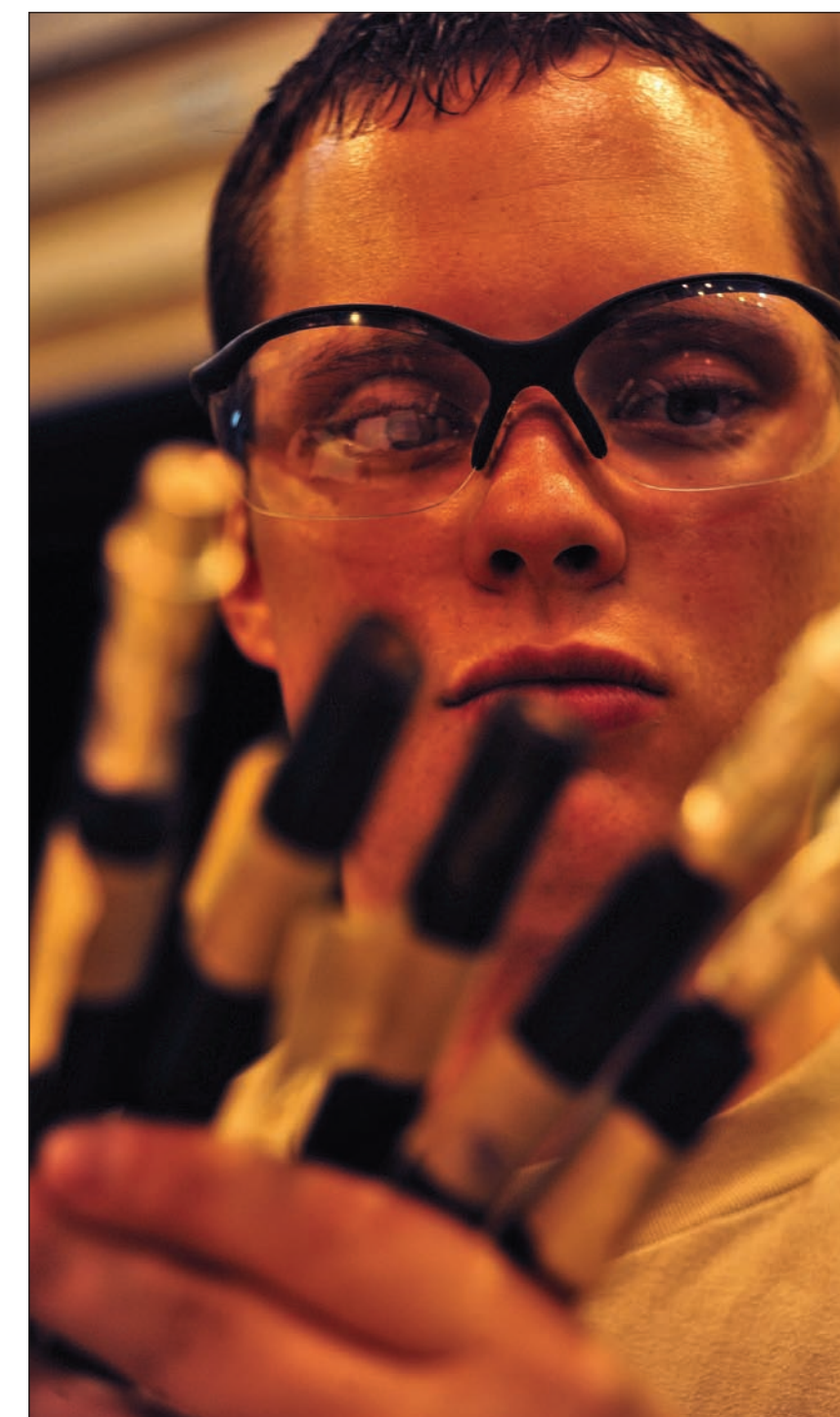
Airman 1st Class James McQueen, 509th Maintenance Squadron Aerospace Ground Equipment apprentice, examines cable heads that provide power to a MHU-204 Munitions Lift Trailer before performing maintenance May 31.
