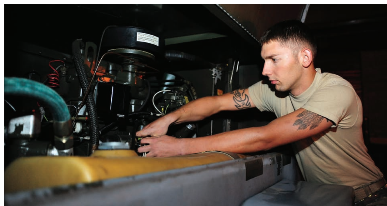
Senior Airman John McLaughlin, 509th MXS Aerospace Ground Equipment journeyman, checks belt tension on an MC-6 diesel engine during a service inspection May 31.
