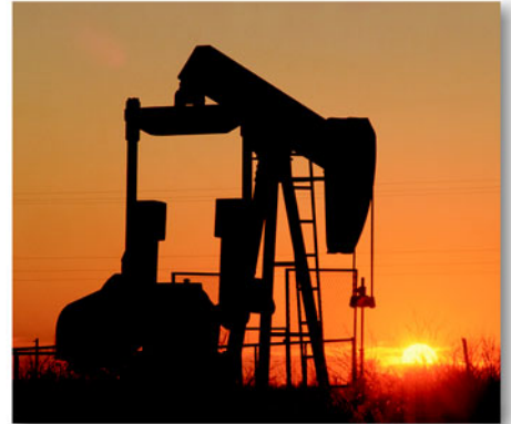
A horsehead pump is used to extract crude oil from a well. This type of pump can lift oil 10,000 feet or more.
