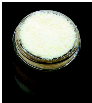
Solidified Mixed Waste Oil After Nochar Treatment
