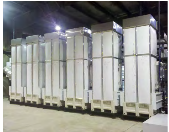
The AltelaRain® 600 turns flowback water resulting from shale gas production into rain-water quality
