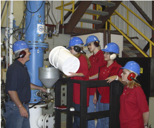
Students load polyethylene beads into a cold flow simulator.
