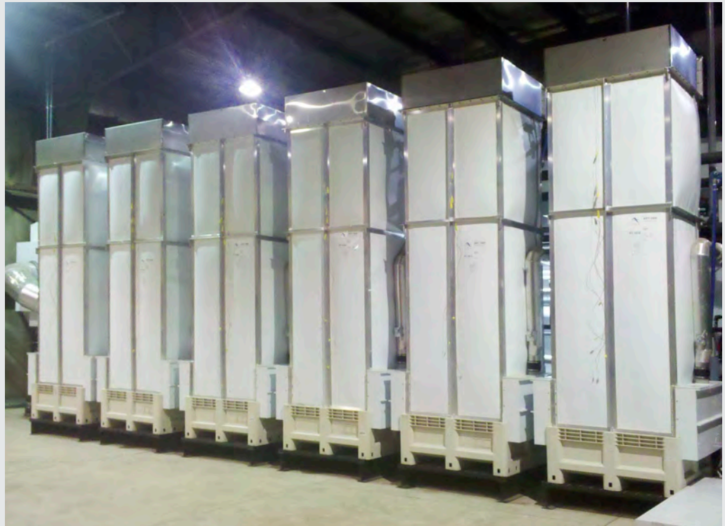
AltelaRain® 600 unit module and water treatment towers.
