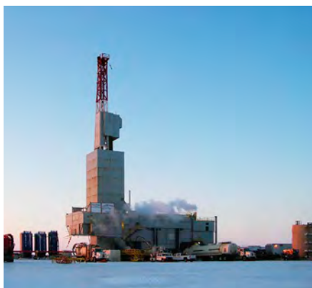
The drilling rig on the site of the DOE-ConocoPhillips "Ignik Sikumi" gas hydrate field trial well in the Prudhoe Bay Unit (Alaska North Slope). In 2011, the well confirmed the presence of multiple underground reservoirs bearing gas hydrate, collected detailed geologic information, and installed an array of down-hole well monitoring devices in advance of production testing operations scheduled to occur in early 2012.
