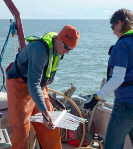
In cooperation with DOE, USGS researchers deploy a mini-sparker source to image seafloor sediments in Alaska's Beaufort Sea.
