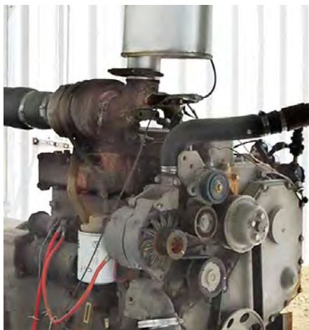
Test engine at Kansas State University's National Gas Machinery Laboratory has been used to evaluate new retrofit technologies for emissions control. (Image courtesy of Kansas State University)
