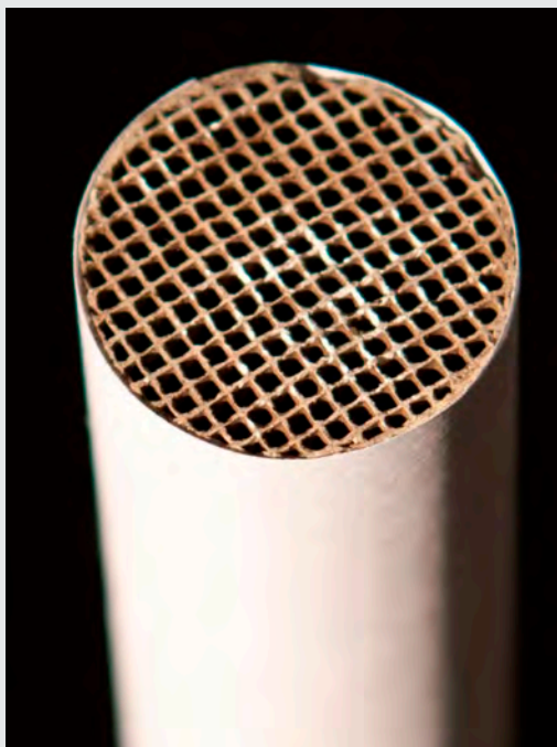
A close-up of a monolith structure that will be coated with NETL's pyrochlore catalyst to reform diesel fuel into syngas.
