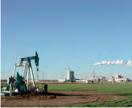
In 2010, NETL demonstrated carbon dioxide flooding EOR in the Hall-Gurney field in Russell Kansas, using carbon dioxide recovered from a nearby ethanol plant. (Image courtesy of Martin Dubois, Kansas Geological Survey)
