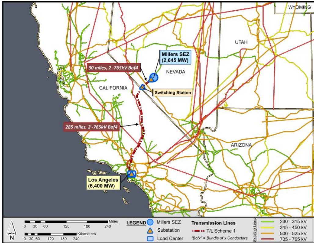
FIGURE 11.7.23.1-2 Transmission Scheme 1 for the Proposed Millers SEZ (Source for background map: Platts 2011)
