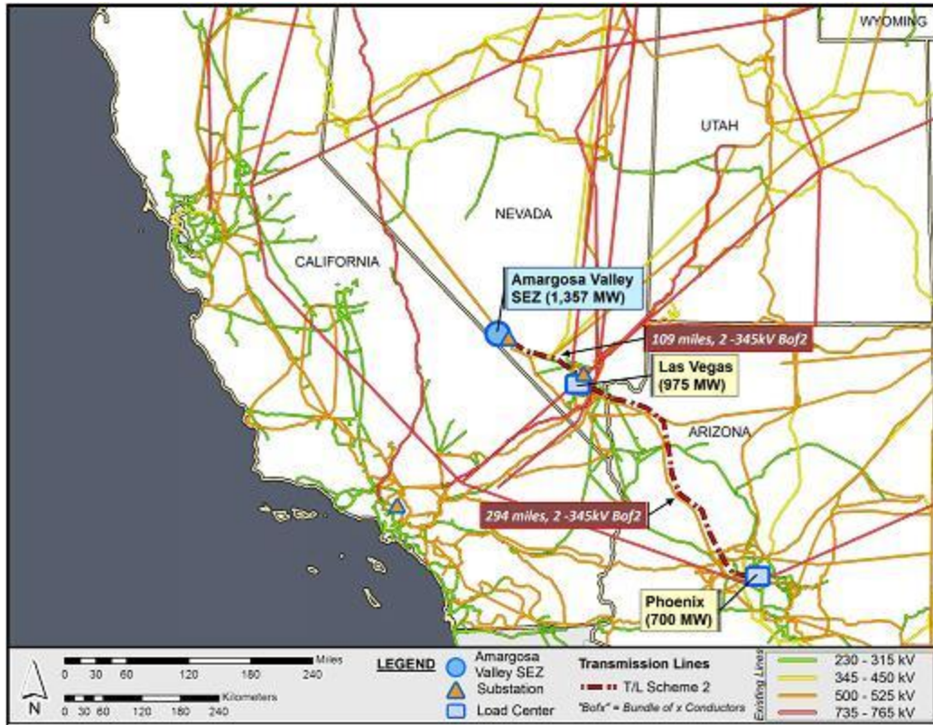
1 2 FIGURE 11.1.23.1-3 Transmission Scheme 2 for the Proposed Amargosa Valley 3 SEZ (Source for background map: Platts 2011) 4 5
