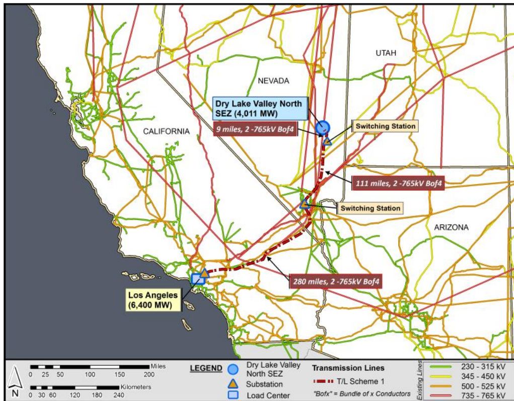
1 2 FIGURE 11.4.23.1-2 Transmission Scheme 1 for the Proposed Dry Lake Valley 3 North SEZ (Source for background map: Platts 2011) 4 5
