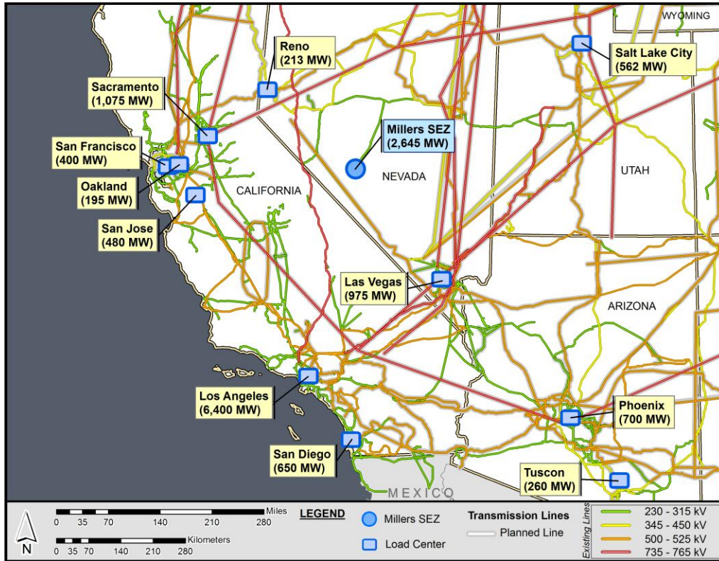
1 2 FIGURE 11.7.23.1-1 Location of the Proposed Millers SEZ and Possible Load 3 Areas (Source for background map: Platts 2011)
