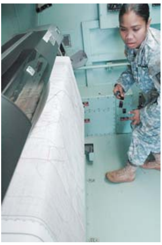
Pfc. Carla Rudimch, 70th Engineer Company, Topographic, checks the High Velocity Map Plotter as it prints a map of the National Training Center, Fort Irwin, Calif.
