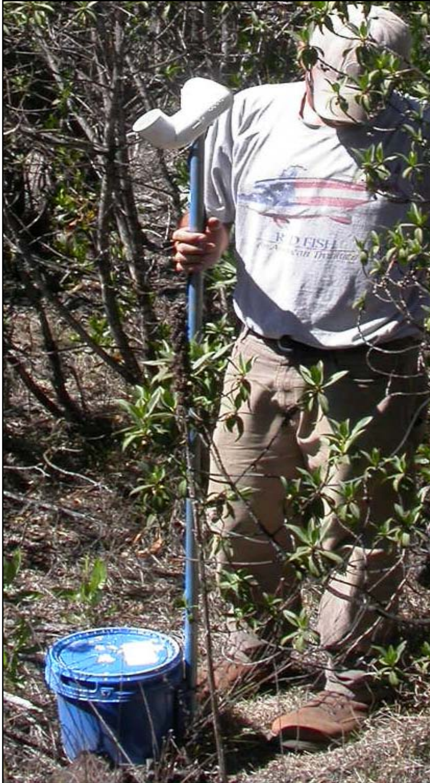
Figure 3.4-3. HHB Automated Detector with Weather-proof Housing Design
