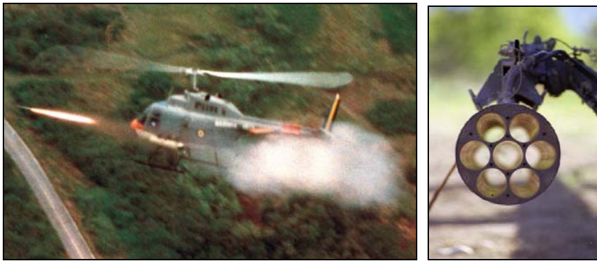
Figure PD 26. Example of 2.75-caliber rocket being fired from a helicopter and 2.75-caliber (70 mm) rocket pod mounted on the side of a helicopter. Unlike the rocket being fired in the photograph, rockets fired at Makua will only be fired from helicopters with nose-down angles of 10 degrees or more.
