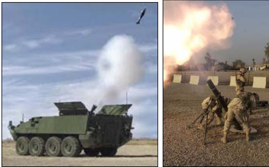
Figure PD 18. The 120 mm mortar may be fired from Stryker or other vehicles or from the ground using a mortar plate (Photos: Global Security.org).
