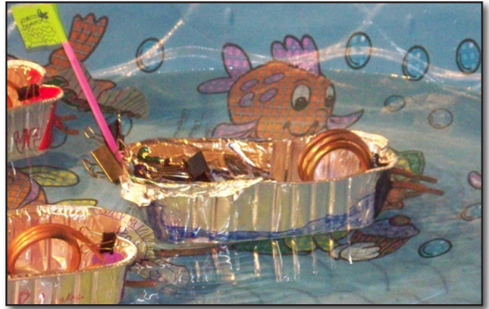
Except for their copper coils, the steamboats were constructed of materials found in most homes, such as light aluminum pans, straws, and binder clips. NIEHS facility staff helped Janoshazi bend the copper pipe to prevent it from crimping. (Photo courtesy of Willis Page)
