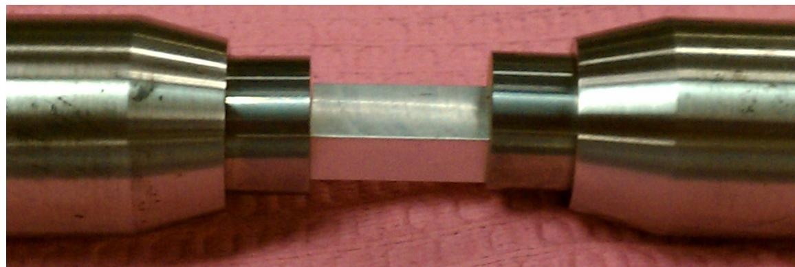
**Compression-MTS-Room-2, MTS loadframe, load level <100kN, compression**
