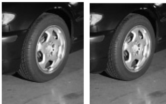
Above: Can you tell which tire is 30 percent under-inflated? Here's what they would look like in the morning, parked in your garage. Tough to tell, isn't it? Tire pressure must be checked with a quality gauge because the pressure cannot be accurately estimated through visual inspection. The tire on the left is under-inflated.
