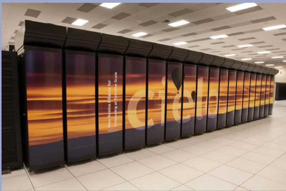
SAFE, SECURE, EFFECTIVE NUCLEAR STOCKPILE : Cielo, currently ranked number 10 in the world with a peak performance of 1.03 petaflops, was recently authorized to conduct classified operations for NNSA. See pages 4 and 5 for more on NNSA's important investment in the future.
