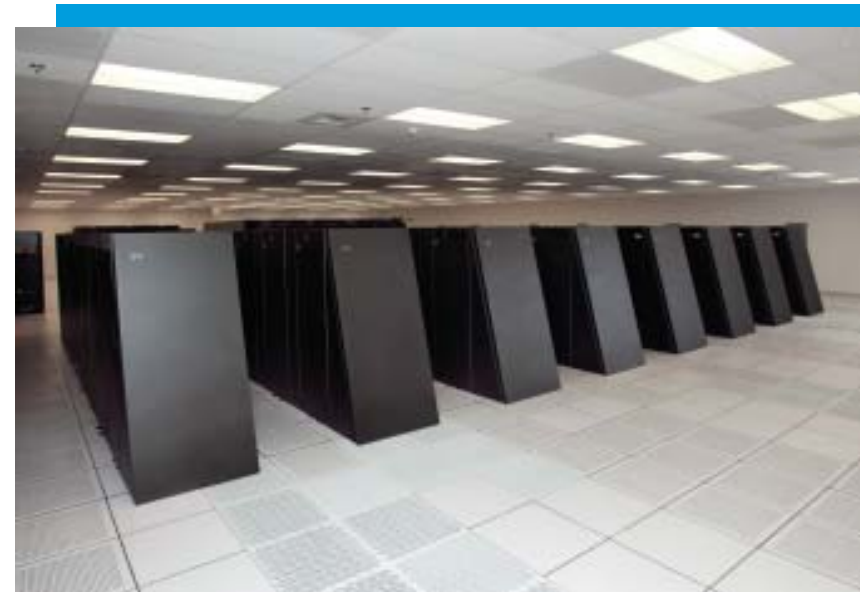
BLUEGENE/L: A revolutionary, low-cost machine delivering extraordinary computing power for the nation's Stockpile Stewardship Program, BlueGene/L entered the Top 500 supercomputer list in November of 2004 and, following life extensions, is currently number 12 with a peak speed of 596 teraflops.
