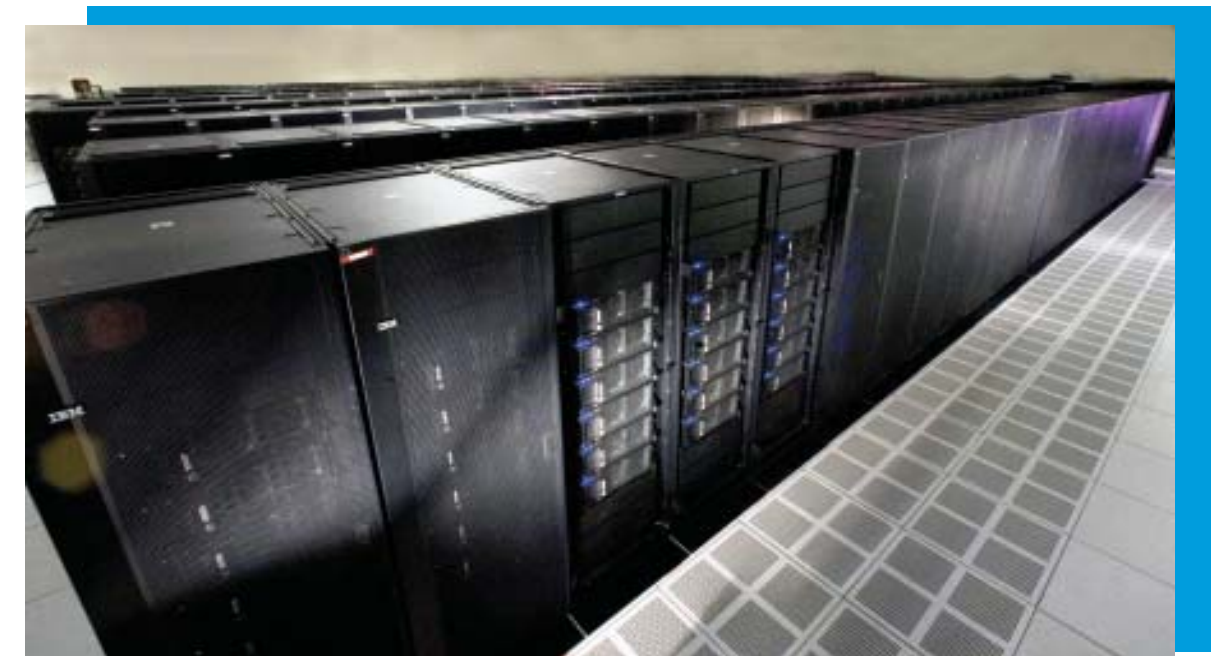
ROADRUNNER: Built by IBM, Roadrunner is currently ranked as the seventh fastest supercomputer. It has a peak performance of 1.38 petaflops, and was the first supercomputer in the world to perform a sustained petaflops calculation. It is also the fourth-most energy-efficient supercomputer in the world on the Supermicro Green500 list.
