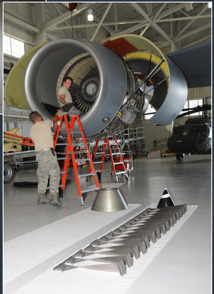
(Right) Tech. Sgt. Jeremy Ascherl hands a first stage fan blade to Master Sgt. Al Schwaderer after removing it from the CFM-International F108-CF-100 turbofan engine on a KC-135 in the Main hanger at Sioux City, Iowa Air National Guard Base. USAF Photo Master Sgt. William Wiseman.
