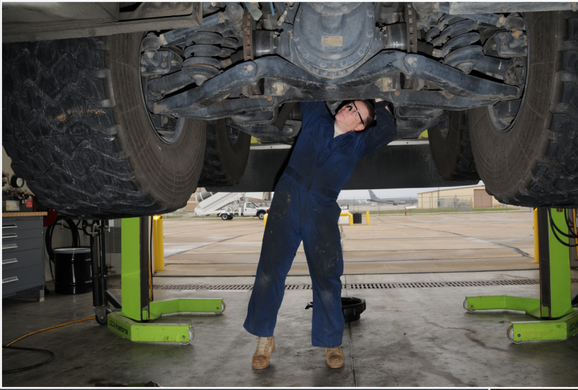
Master Sgt. Neal Stokes, 185th Air Refueling Wing (ARW) vehicle maintenance, works on a fire truck at the 185th vehicle maintenance shop in Sioux City, Iowa. The large vehicle is raised using specially designed hoists to allow periodic maintenance. USAF Photo Master Sgt. Vincent De Groot
