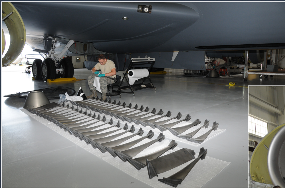
(Above) Staff Sgt. Ben Weins, 185th Air Refueling Wing aircraft jet engine mechanic, cleans the first stage fan blades from the engine of a KC-135 prior to a 1500 hour inspection in the main hanger at the Sioux City, Iowa Air National Guard base on June 27, 2011. The blades are inspected every 1500 hours of run time. USAF Photo Master Sgt. William Wiseman.
