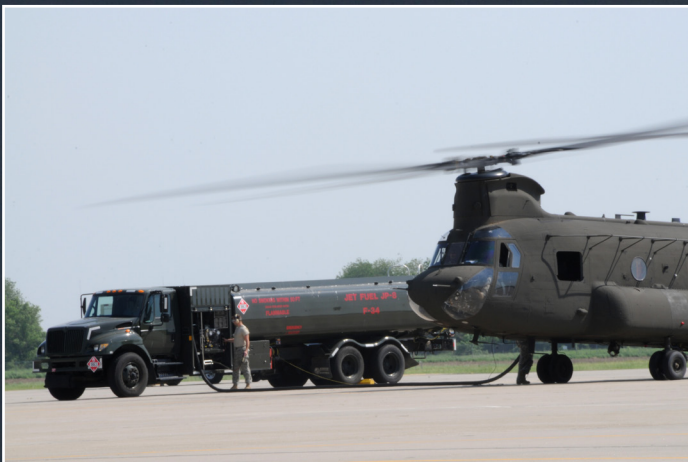
A CH-47 Chinook helicopter, from Company B, 2nd Battalion 238th Aviation, based in Peoria Illinois, is being refueled while on the ramp at the Iowa Air National Guard base in Sioux City, Iowa. Members of the 185th Air Refueling Wing based in Sioux City are refueling the helicopter while it is still running. "Hot Refueling" saves time for the air crew who will return to flooded areas along the Missouri River. National Guard Soldiers from Minnesota, South Dakota, Illinois and Iowa assisted local and state authorities in Western Iowa and South East South Dakota to protect private properties and municipalities along the swollen Missouri River.
