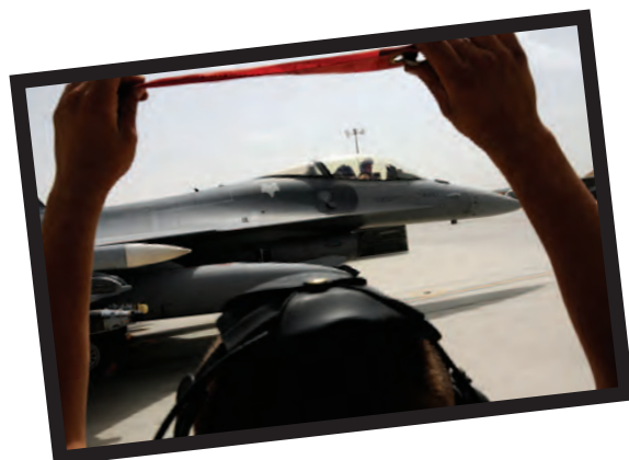
Airman 1st Class Robert Barber, a crew chief, shows Captain Jerrod Sonderman the EPU pin has been pulled as he prepares to launch an F-16 fighter jet for a mission, May 30, 2012.
