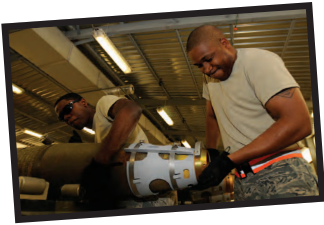
Airman 1st Class Rahkeem Jenkins and Staff Sgt. Symeon Graham, ammo technicians, install tail and nose fuses on a GBU-38 bomb, April 21, 2012.
