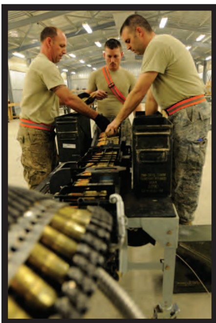
Senior Airman Tony Goodwin, Airman 1st Class Benjamin Lawrence and Tech. Sgt. Robert Seter, conventional munitions maintainers, reload 20mm rounds, used in F-16 Fighting Falcons, to the Universal Ammunition Loading System, June 9, 2012
