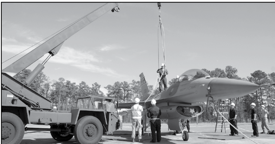
Crew chiefs with the 169th Aircraft Maintenance Squadron respond to a simulated aircraft mishap with a F-16 and UH-60 Black Hawk helicopter. The F-16 is connected to a crane to be transported from the accident sight.
