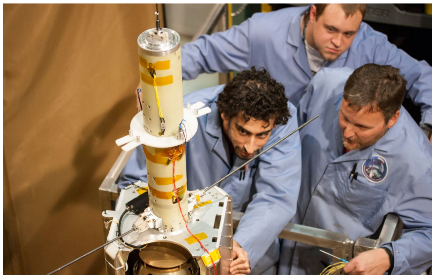
Paul, Brian and Nate investigating the boom latching mechanism.
