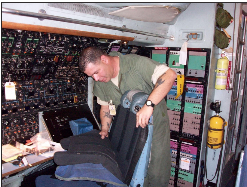
Master Sgt. Rick Fujimoto, a crew chief with the 653rd Combat Logistics Support Squadron, installs battle armor to the pilot's seat of a C-5 Galaxy. Sergeant Fujimoto is the armor installation team leader overseeing 445th Airlift Wing's C-5 armor installation process. (Courtesy photo)
