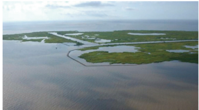
Aerial view of the east end of Marsh Island where material dredged from East Cote Blanche Bay will be deposited to fill in open ponds and nourish marsh.
