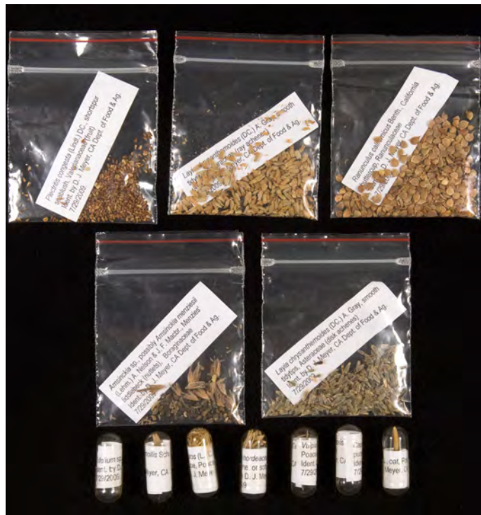
Figure 8 Example of the main content of a specimen, after identification, placed in one or more individual small zip bags and “contaminating” species placed in individual gelatin capsules
