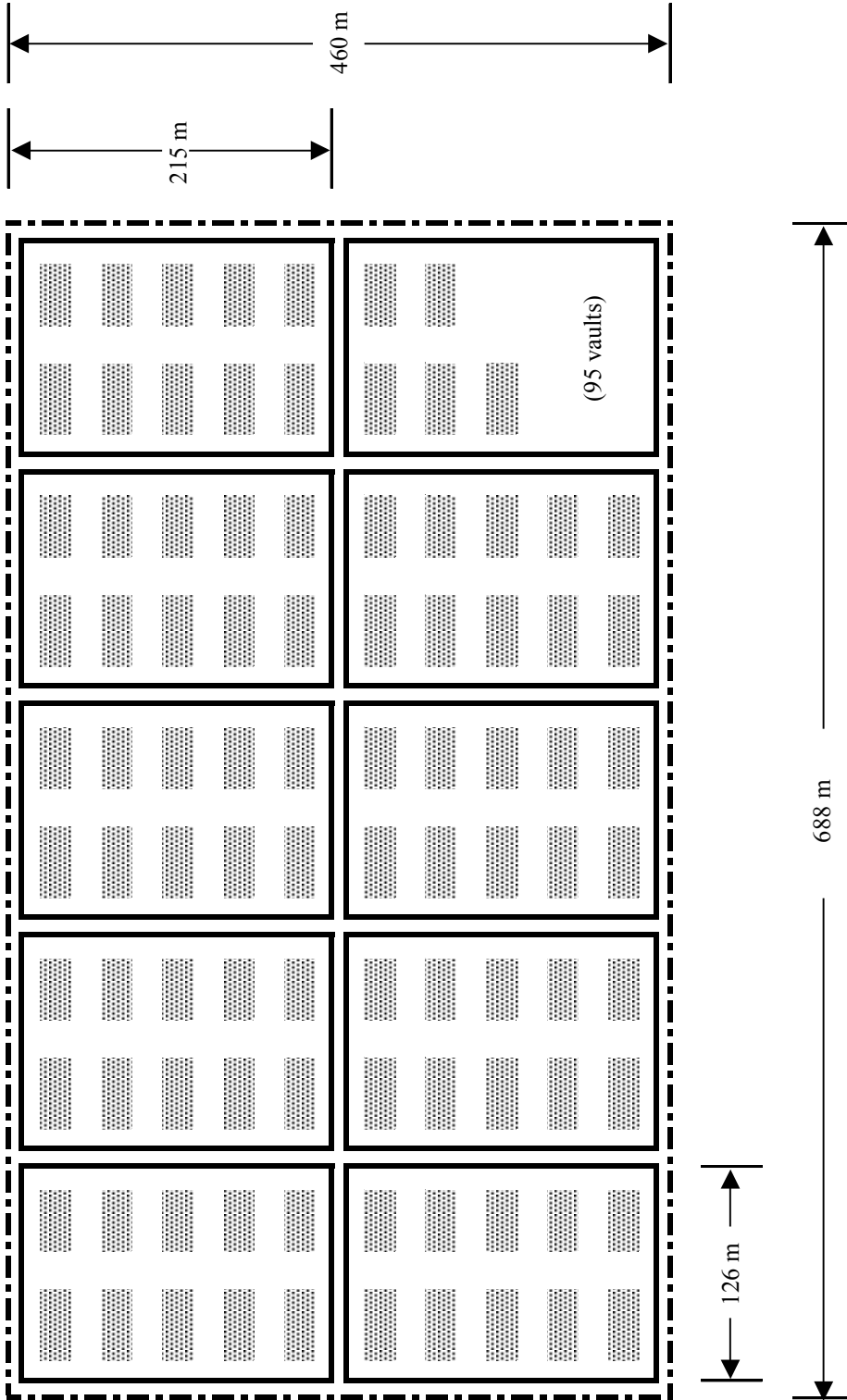
FIGURE 3.2a Site Map for Construction of the Vault Disposal Facility: New Inventory, 30-Gallon Drums (not to scale)
