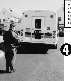
With the engine running, turn on all the lights - headlights (low and high beams), parking lights, brake lights, turn signals, emergency flashers, back-up lights, clearance lights and interior lights.
