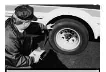
Check for proper tire inflation and any cuts, bubbles or other tire deformities.
