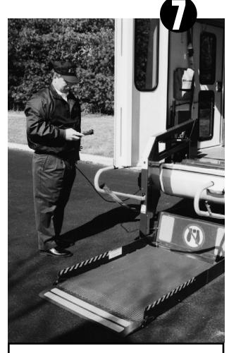
Cycle the wheelchair lift and check that all of its securements are present and working properly.
