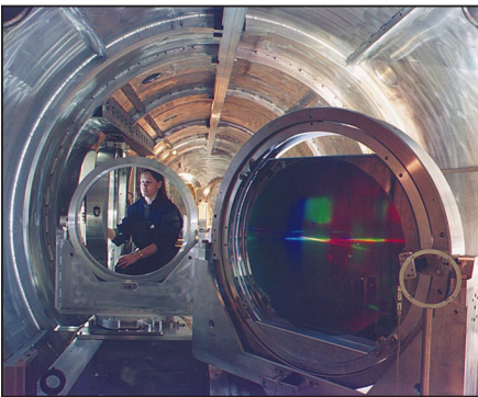
This pair of large gratings inside a vacuum compression chamber at the output of Nova was used to produce a petawatt (million-gigawatt) laser output pulse in 1996.
