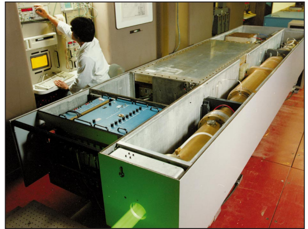
A copper vapor laser amplifier is undergoing testing in an LLNL facility.
