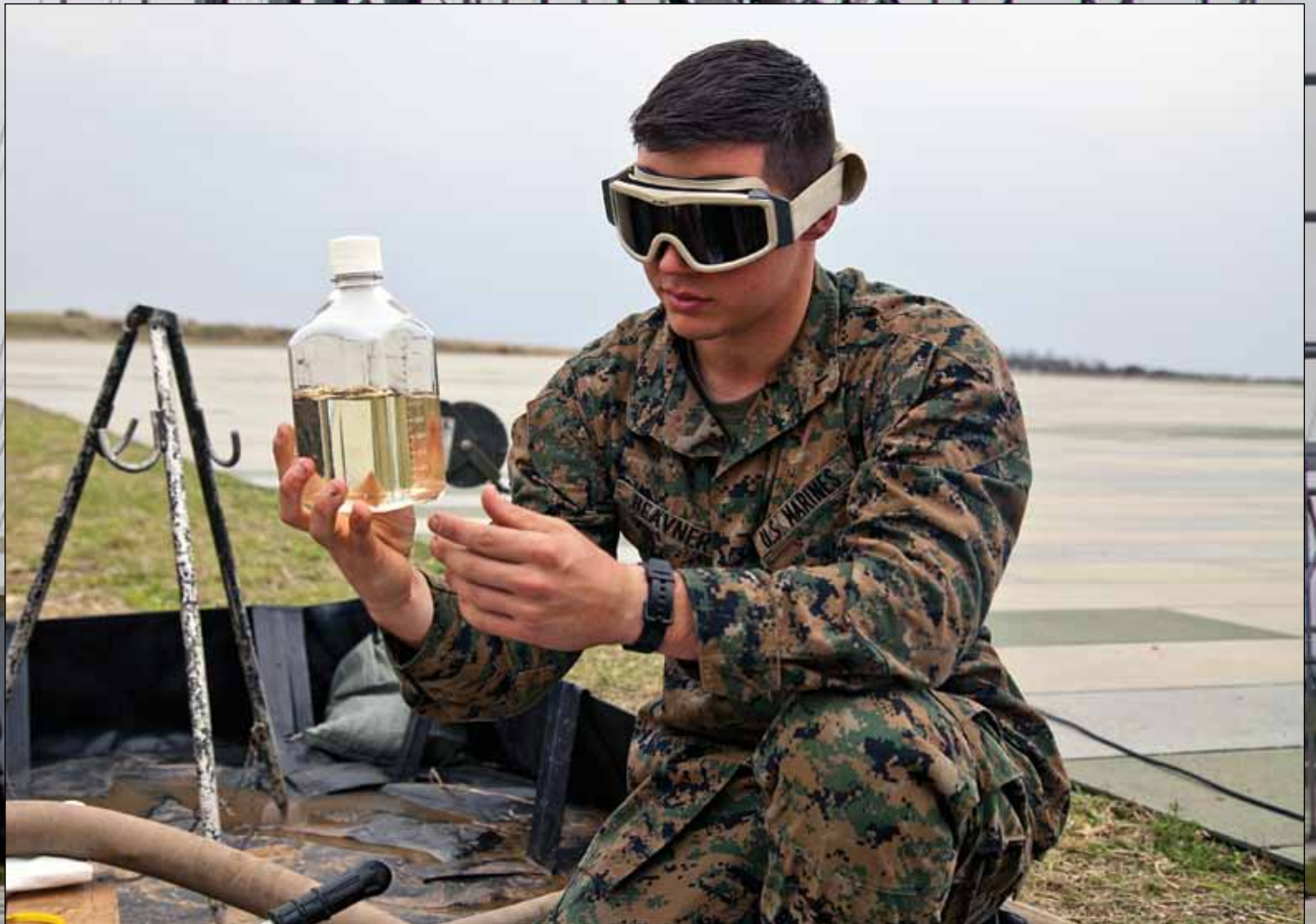
Pfc. Colby J. Heavner takes a fuel sample during bulk refueling training Jan. 16 at Ie Shima training facility. The samples are used to test the fuel potency and check for contaminants to ensure the aircraft receive high-quality fuel. Heavner is a bulk fuel specialist with Marine Wing Support Squadron 172, Marine Aircraft Group 36, 1st Marine Aircraft Wing, III Marine Expeditionary Force.
