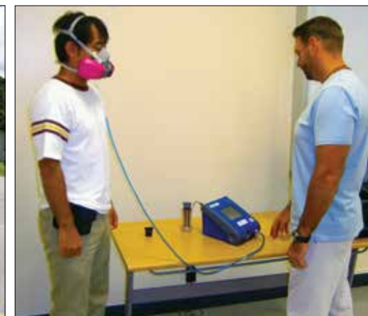
A respiratory protection program manager performs a qualitative fit test of respiratory protection on a Marine Corps Base employee. 海兵隊基地従業員のマスクの品質テストをする呼吸器保護プログラム責任者。Photos courtesy of Marine Corps Base Camp Butler Installation Safety Office
