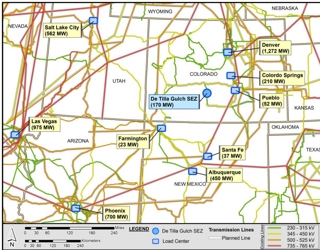
FIGURE 10.2.23.1-1 Location of the Proposed De Tilla Gulch SEZ and Possible Load Areas (Source for background map: Platts 2011)
