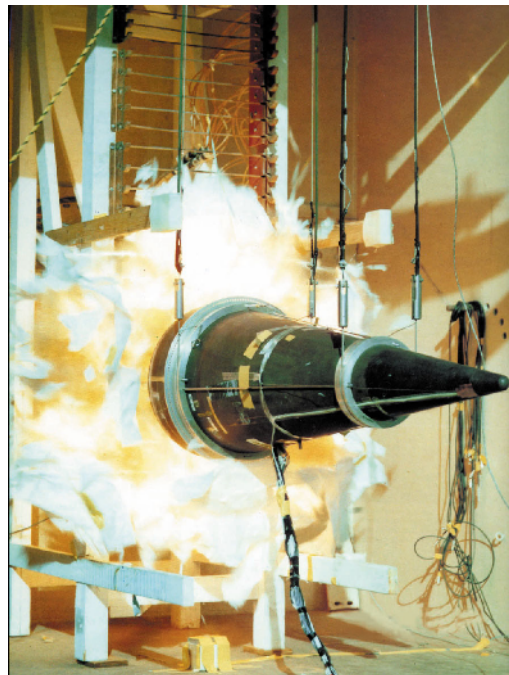
Components of a Peacekeeper missile are subjected to a wall of fire. Such testing helps determine how aging weapons will perform in the future.
