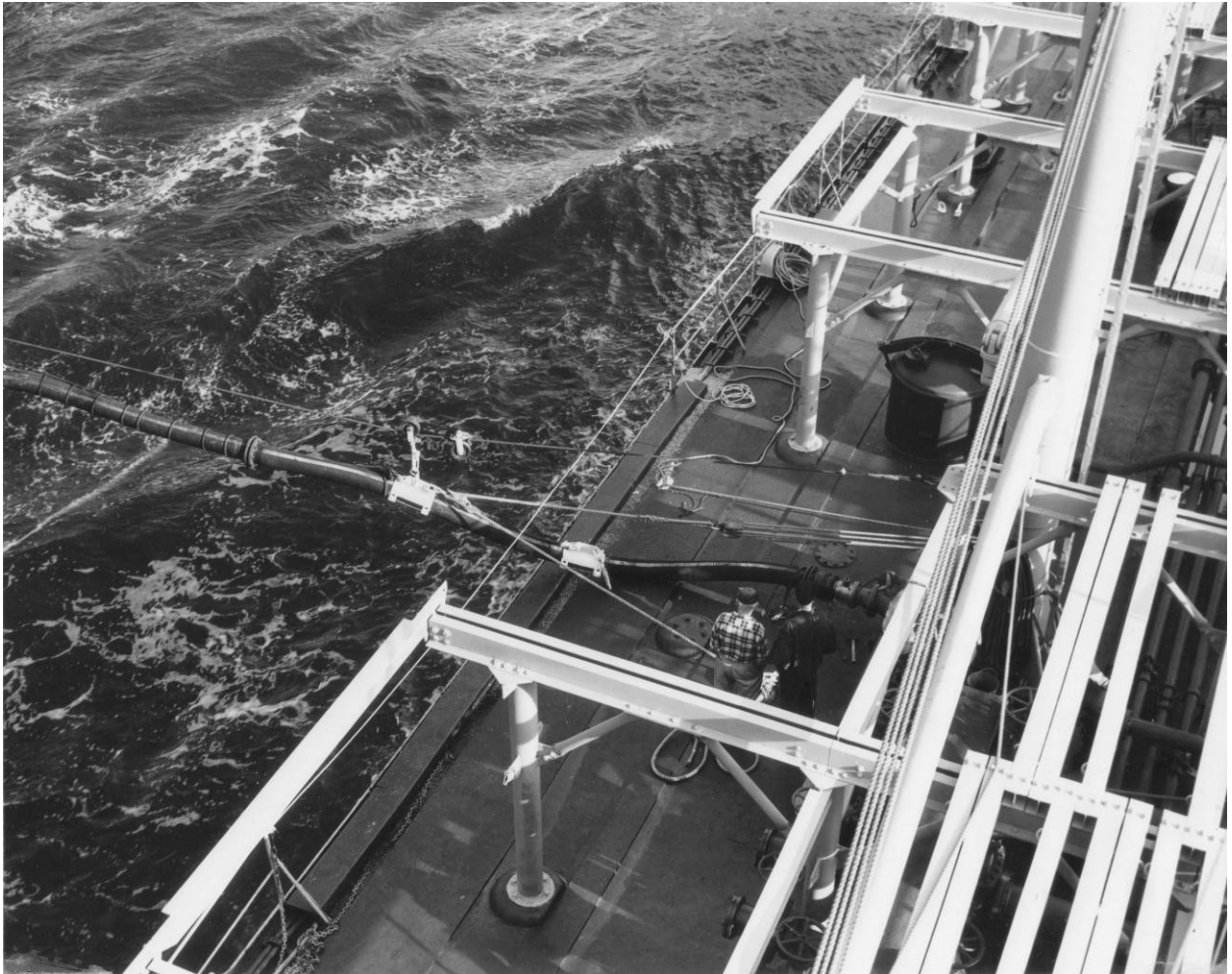
Figure 2: USNS Mission Santa Ynez (AO-134) refueling-at-sea rig. From MSC Files, Naval Historical Center Photographic Section, Washington, DC.
