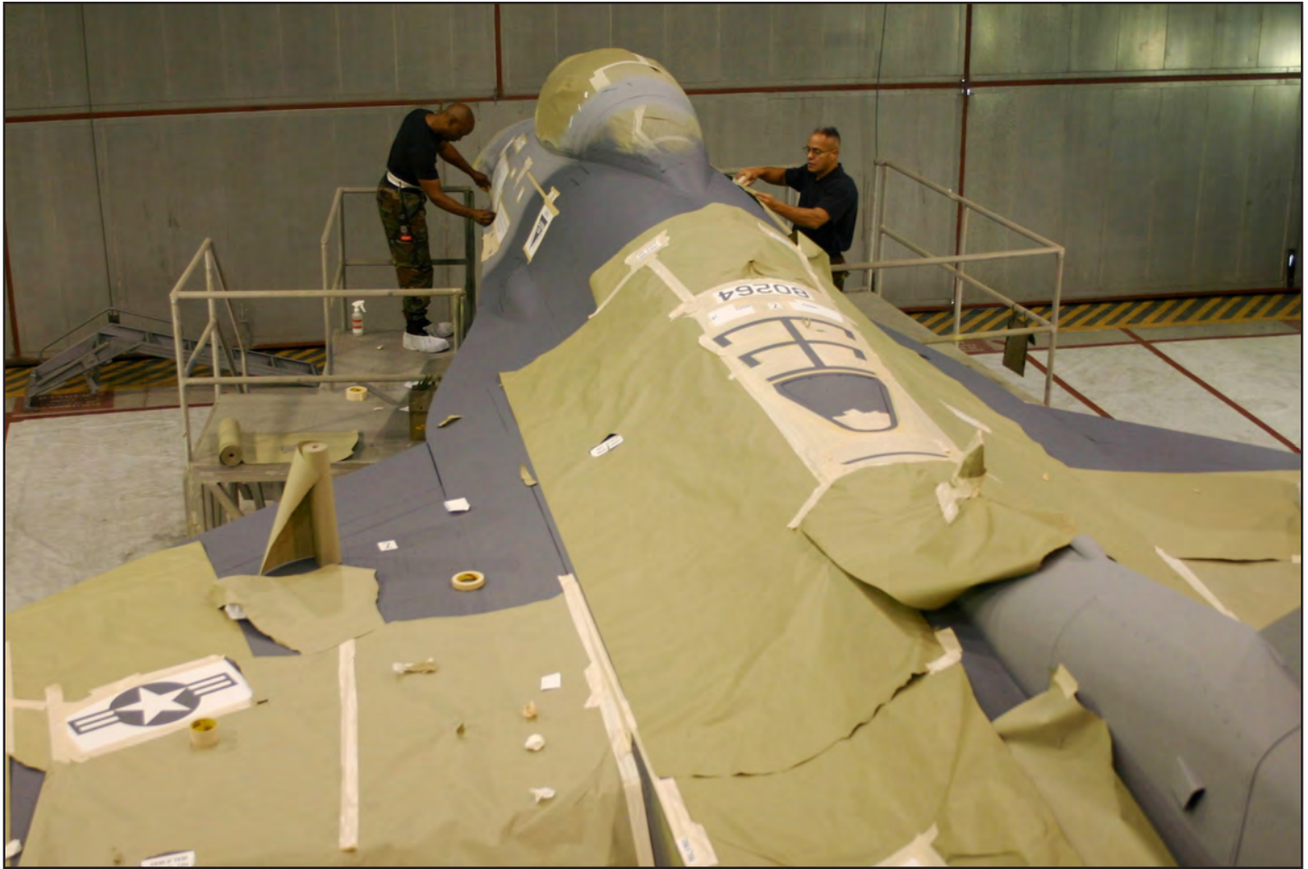
Tech. Sgt. George Walker, left, and Tech. Sgt. Luis Velez, structural maintenance technicians from the 482nd Maintenance Group, prepare stencils on an F-16 prior to painting Nov. 4 here at Homestead Air Reserve Base.
