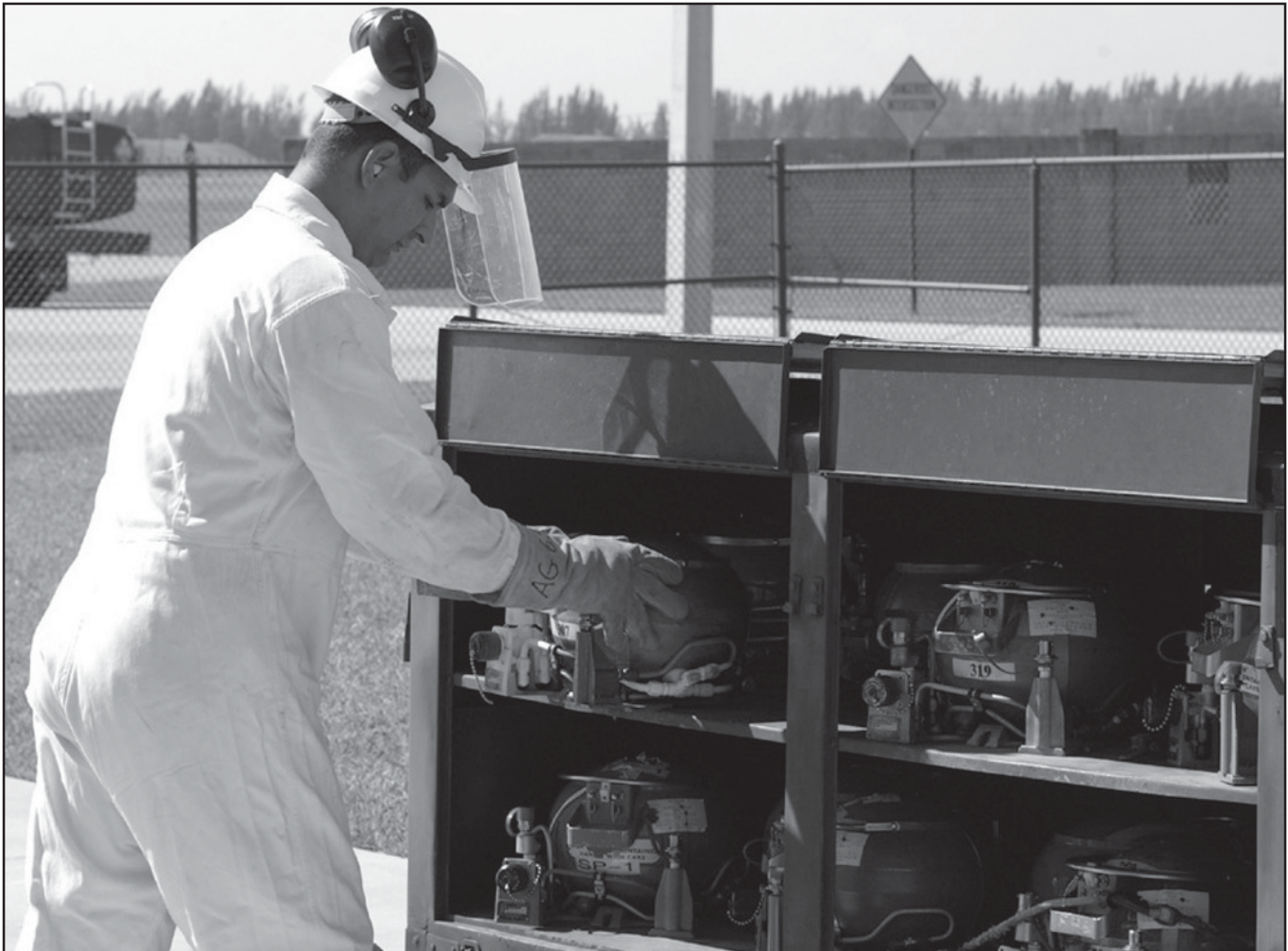
Safety is of utmost importance when handling liquid oxygen. 482d Maintenance Squadron Crew Chief, Senior Airman Sean Powers prevents contact of body oils with oxygen by wearing gloves and using brass tools. Handling oxygen requires three weeks of technical school and three weeks of cryogenics training.
