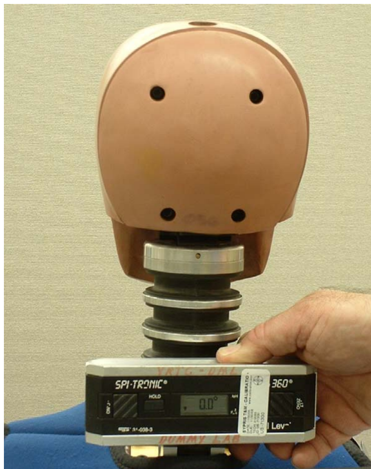
Figure 45. Adjusting the SID-IIIsD dummy in the lateral direction
