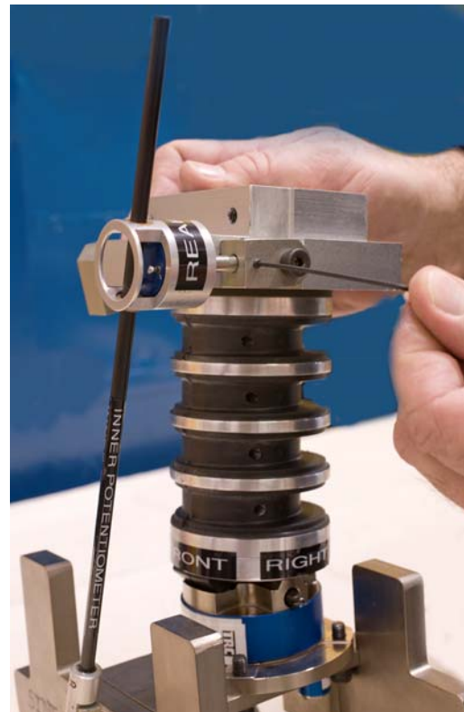
Figure 33. Tighten set screws for inner potentiometer pivot bracket
