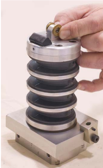
Figure 24. Install brass nodding joint washers
