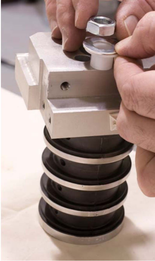
Figure 20. Install lower neck bushing, washer, and hex nut onto neck cable
