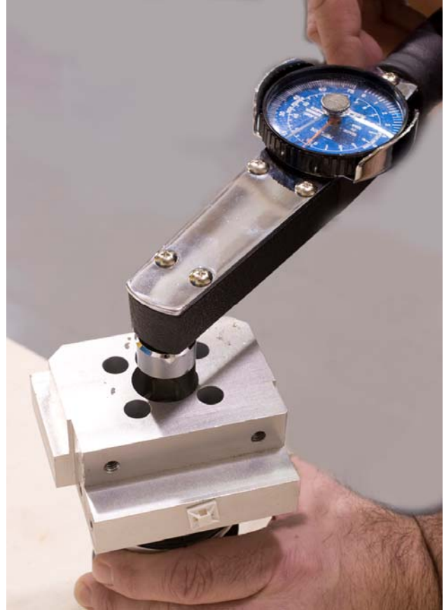
Figure 21. Torque hex nut on neck cable to 10-12 in-lbs
