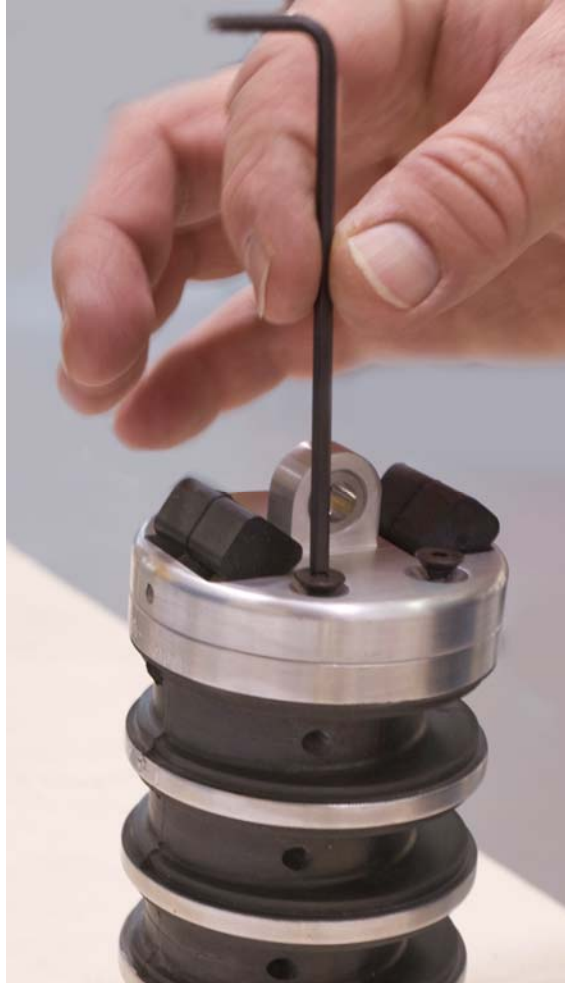
Figure 17. Removing the nodding joint assembly
