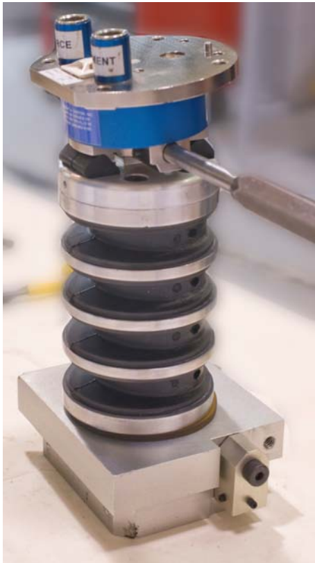
Figure 26. Align brass nodding joint washers with holes
