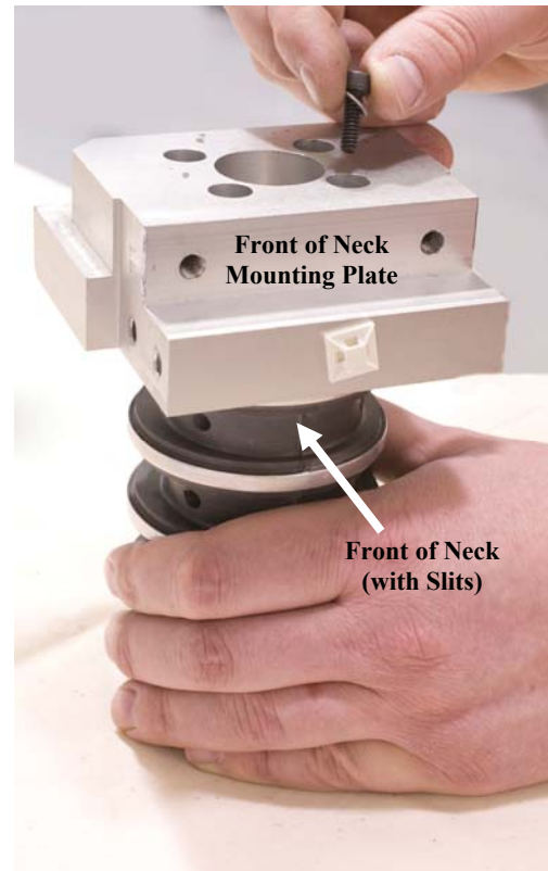
Figure 19. Assemble molded neck to neck mounting plate
