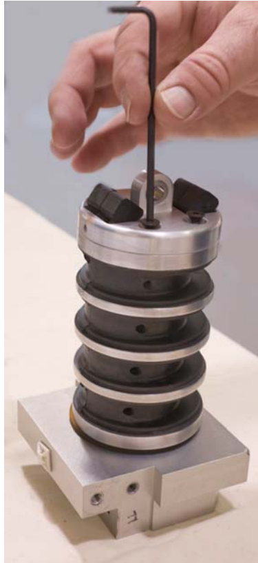
Figure 22. Reinstall neck nodding joint assembly
