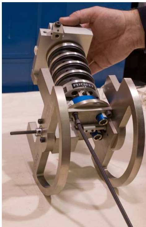
Figure 28. Install upper neck load cell to head form
