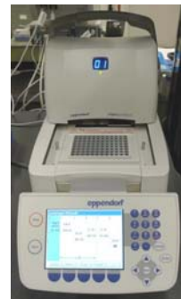
Eppendorf Mastercycler pro Ramp rate = 6°C/sec
