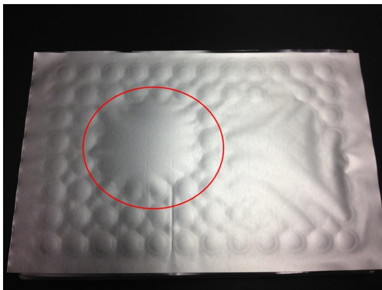
Figure 1.6: Failure in heat seal application
