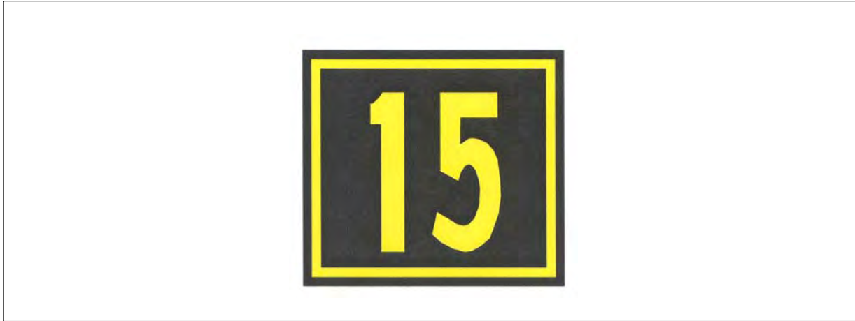
FIG AD 1.1-46 Runway Location Sign
