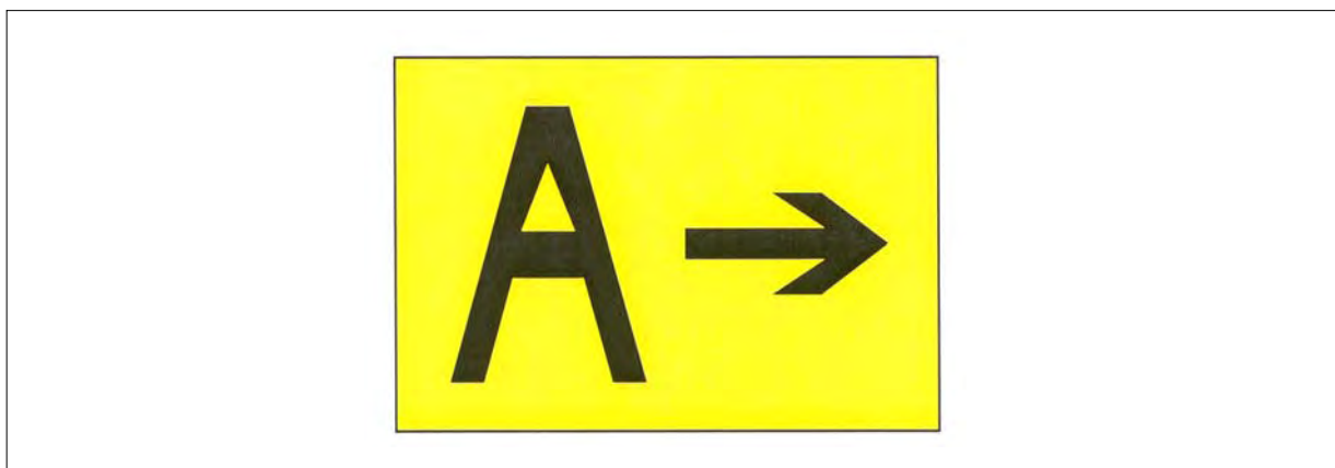
FIG AD 1.1-50 Direction Sign for Runway Exit
