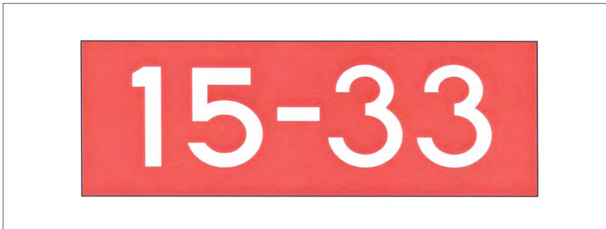
FIG AD 1.1-38 Runway Holding Position Sign
