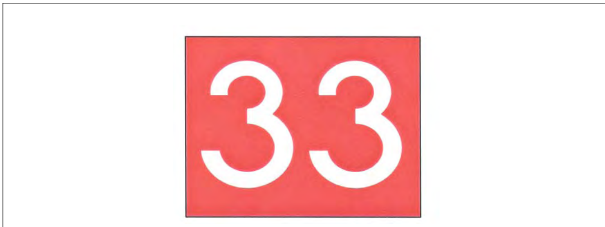
FIG AD 1.1-39 Holding Position Sign at Beginning of Takeoff Runway
