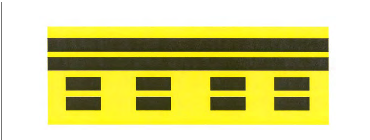
FIG AD 1.1-47 Runway Boundary Sign
