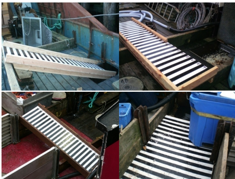
Figure 1. Clockwise from upper left, halibut discard chutes on the F/V Laura, F/V Pacific Star, F/V Excalibur II and the F/V New Life.
