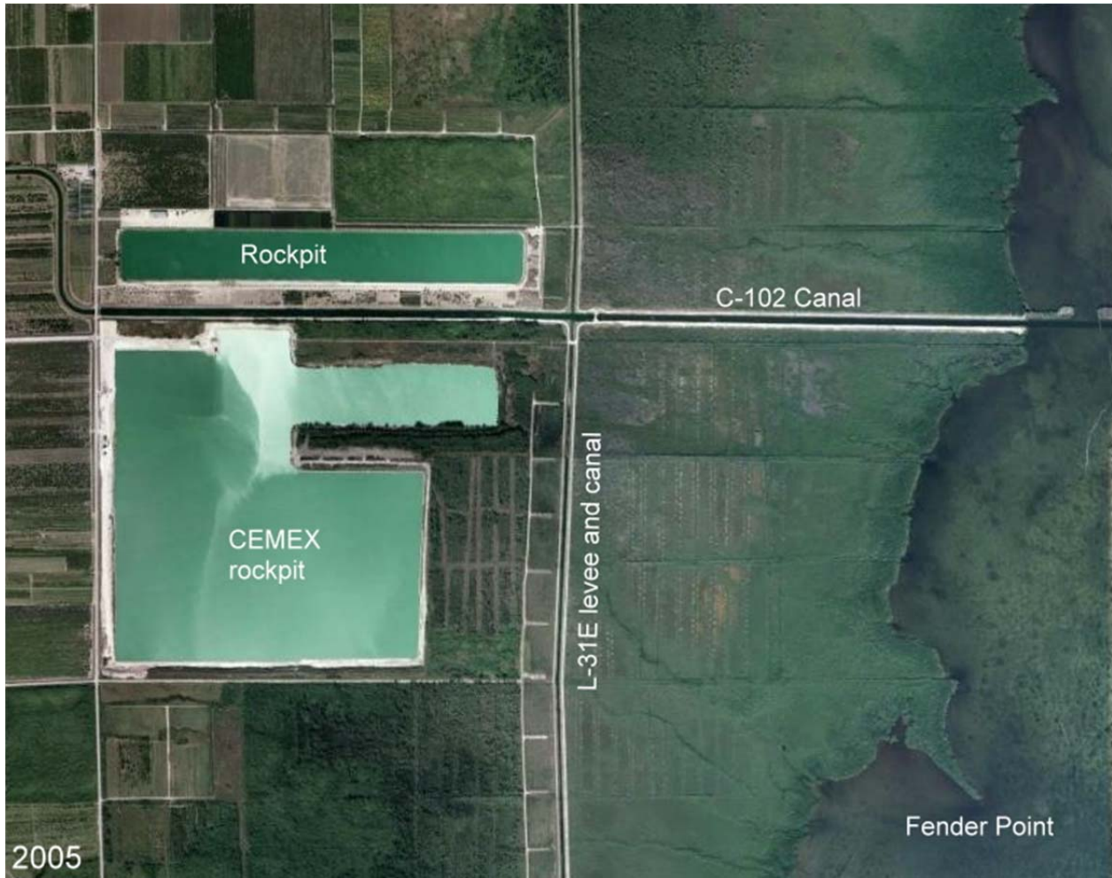
Figure 42. Aerial photo of large limestone mines (rockpits) located just west of the park boundary along L-31E levee. The older northern example is approximately 1,425 x 177 m in dimension; the larger one (owned by CEMEX) is about 1,355 m x 1,165 m and has recently been closed out. Miami-Dade DERM has been monitoring water quality in this pit for some time (FLADOT, 2005).
