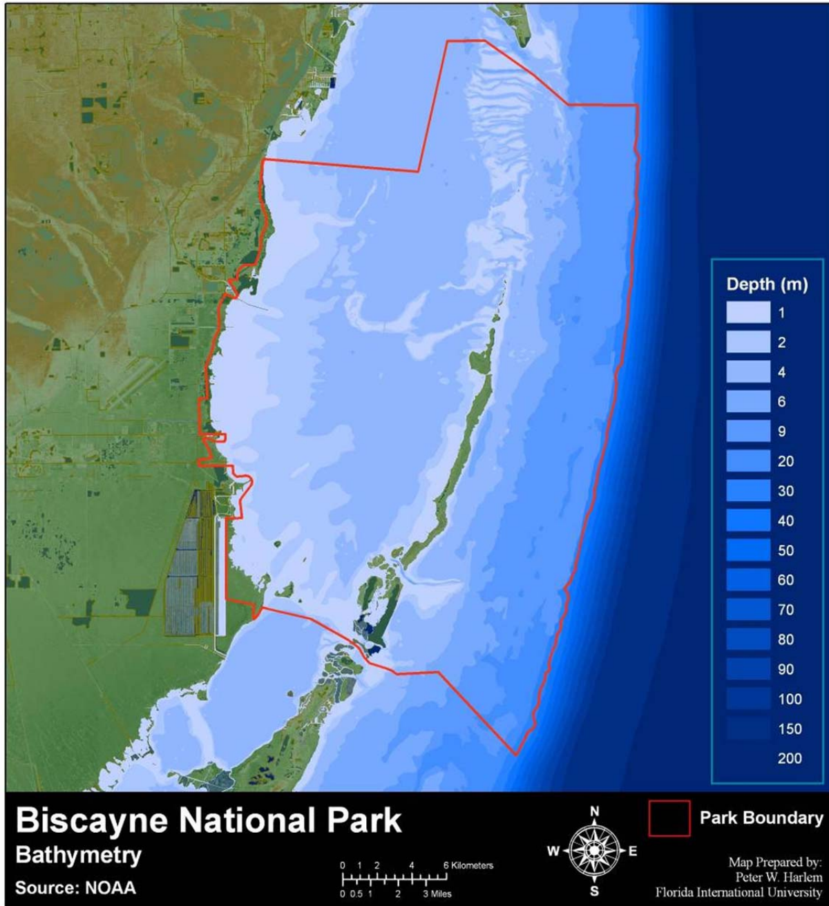
Figure 33. Bathymetry of Biscayne National Park from NOAA nautical charts. The central axis of the bay is uniformly deep, except where crossed by shoal sediments such as at Featherbed Bank. Deeply cut tidal channels bisect the rise formed by the Key Largo Limestone along the trend of the Keys.
