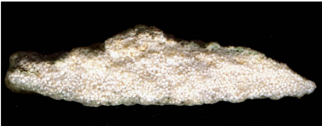
Figure 28. Oolitic facies of the Miami Formation. This slab section shows well-developed clear calcite cement holding the white ooids together, making this particular layer more resistant to weathering. These indurated layers alternate with softer, less cemented ones, and make the cross bedding easy to see in most outcrops of this facies. At the top the ooids have popped out showing the moldic porosity for which the formation is well known (P. W. Harlem).
