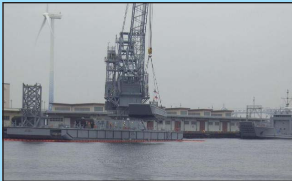
Barge Derrick Crane
