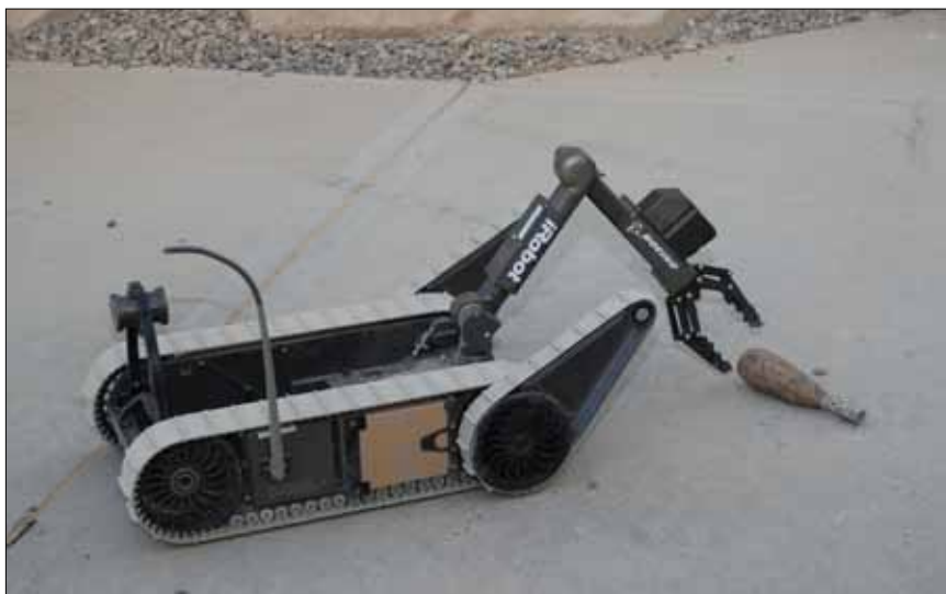
An iRobot PackBot picks up a demonstration object at the Joint Robotics Repair Detachment at Victory Base Complex, Baghdad. The robots can be operated by a commercial off-the shelf controller or a heads-up display.
