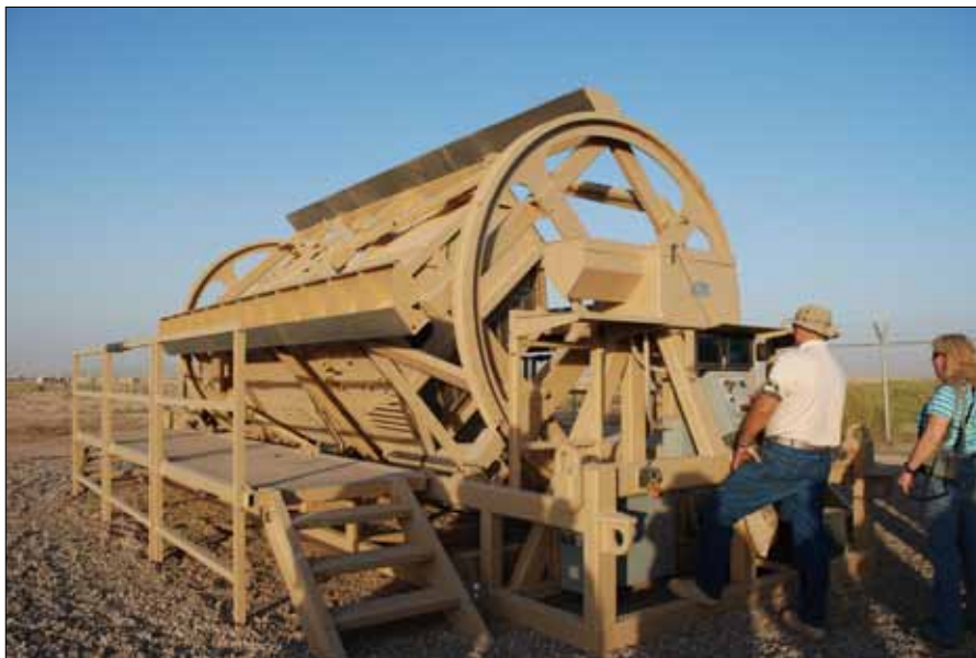
Alan Tiffany, a Raytheon contractor, operates the MRAP Egress Trainer during an officer professional development training session Aug. 19 at Joint Base Balad, Iraq. The device is used to train Soldiers on how to safely exit an MRAP in the event of a roll-over. Fourteen METs have been fielded by the 402nd Army Field Support Brigade Acquisition, Technology and Logistics Directorate. ALT-D has fielded more than 300,000 cutting-edge items to Soldiers on the battlefield.
