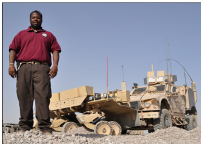
Albert Bacon, service representative for R4 a contractor supporting Product Manager IED Defeat/Protect Force, stands in front of a mine-resistant ambush-protected vehicle with a mine roller attached to it at AFSBn-Kandahar.
