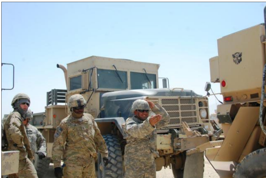
Staff Sgt. LeJaun D. Taylor, a U.S. Army Ordnance School instructor, (center) and Soldiers completing the H8 Additional Skill Identifier course watch Sgt. Thomas J. Smith, E Company 3/10 General Support Aviation Battalion, 10th Combat Aviation Brigade, as he uses hand signals to guide a M1089 five-ton MTV wrecker into position to tow a disabled vehicle.
