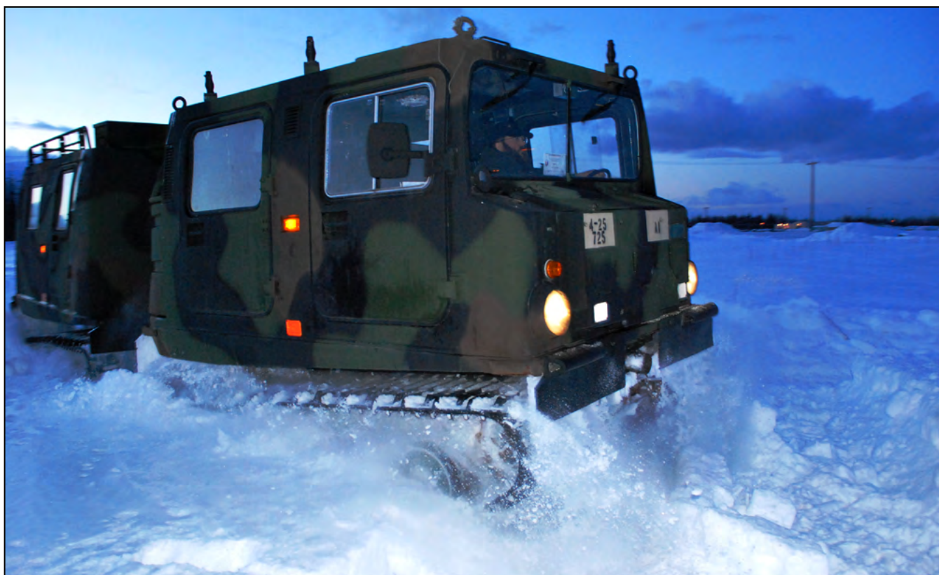
Kent Hubert, automotive equipment specialist, Army Support Activity, Tactical Maintenance, demonstrates the ease of driving a Small Unit Support Vehicle (SUSV) during the morning hours at Joint Base Elmendorf-Richardson, Alaska. The vehicle, which can be used to transport troops, can drive in any depth of snow, making it extremely valuable for emergencies.
