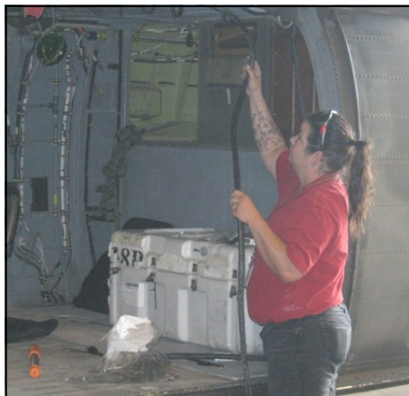
Sara Watrers, an A2C2S FSR runs wire bundle through sound proofing.
