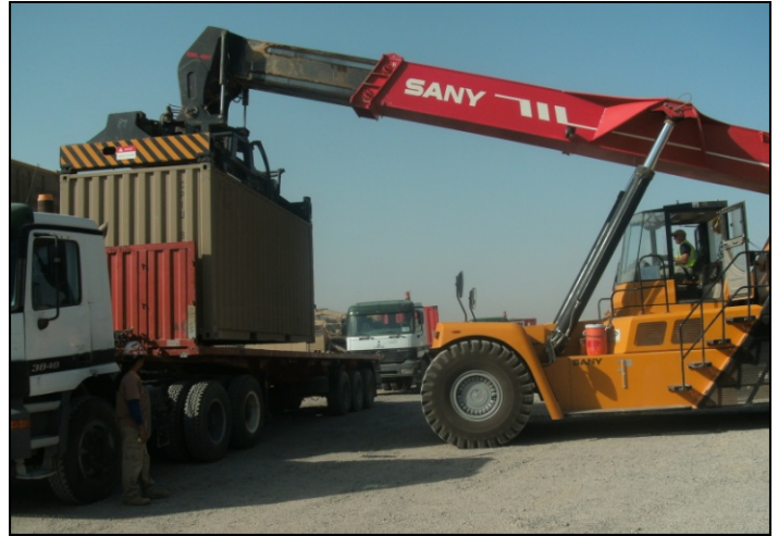
RTCH loading Route Clearance container on trailer.
