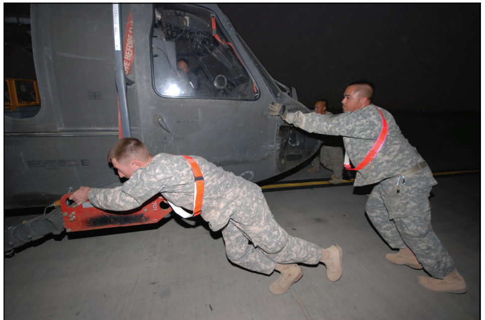
Soldiers from the 25th CAB push a UH-60 Blackhawk into place so it can be winched aboard an Air Force C-17 Globemaster.
