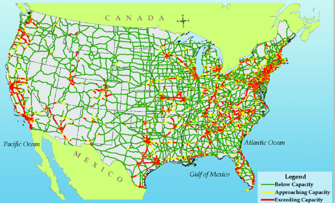
Figure 3-3. National Highway System Estimated Peak Period Congestion: 2020
