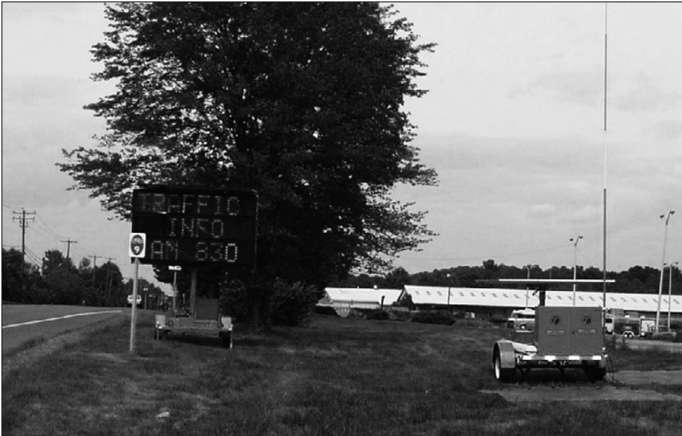
Figure 17. Portable DMS and Portable HAR Unit at the Dutchess County Fairground
