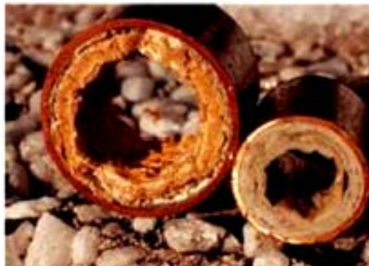
Figure 7: Example of Pipe Scaling
