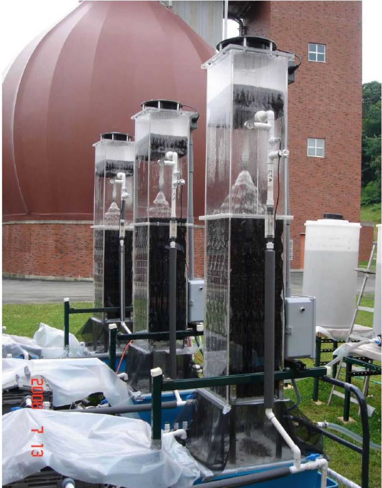
Figure 9: Pilot Scale Cooling Towers in Operation at the Franklin Township Municipal Sanitary Authority
