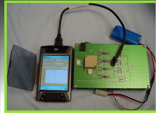
Figure 1: Acoustic wave biosensor instrument with PDA controller and rechargeable battery. Sensor arrays fit in the tan enclosure on the circuit board.
