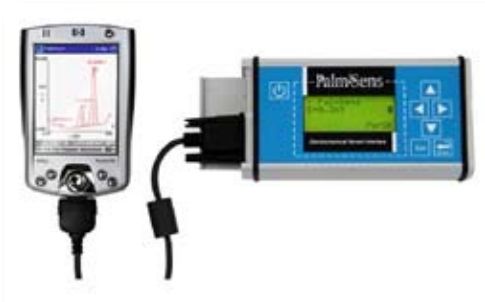
Fig. 6 Photograph of PDA-controlled potentiostat for use with ElectroNeedle™ array.
