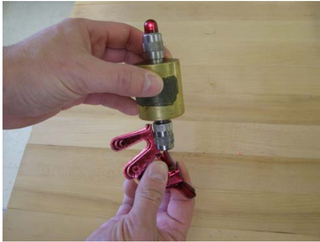
Figure 8 – Sharp Point Test
