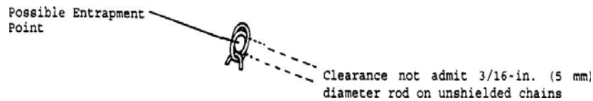
Figure 43 Chain Link Clearances
